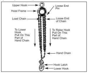
Operate the hoist with no load and then a light load of approximately 50 pounds (23 Kg.) times the number of load supporting chains to make sure it operates properly and the brake holds the load when the hand chain is released; then operate with a rated load as shown on the capacity plate.
